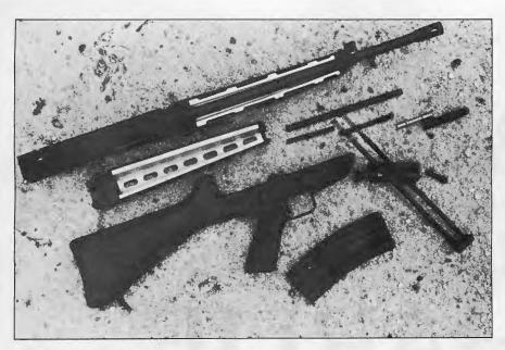
SAR 80 rifle disassembled.
